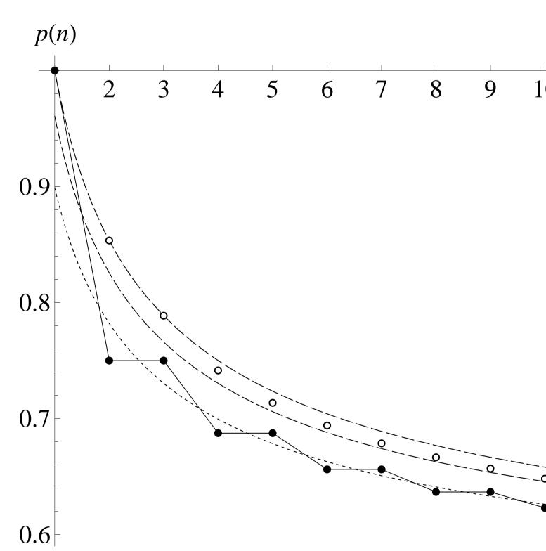
Success probabilities of classical and quantum RACs with SR. Black dots correspond to optimal classical RAC with SR and dotted line shows the asymptotic behavior. Circles correspond to numerical QRACs with SR and dashed lines to quantum upper and lower bounds, respectively.
